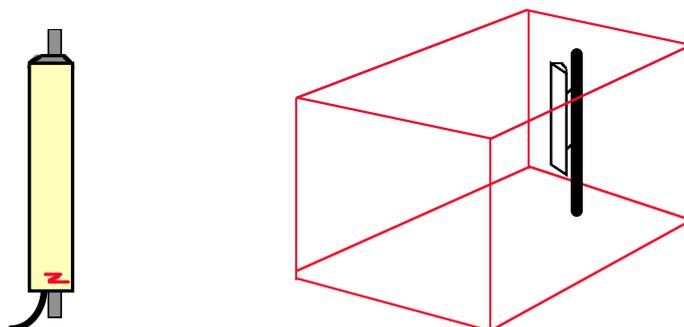
The signals from mobile telephony sector antennas form a rectangular exclusion zone which extends above, below and behind the antenna as well as to the front and sides.
