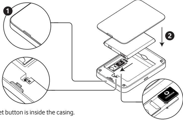
Reset button is inside the casing.
