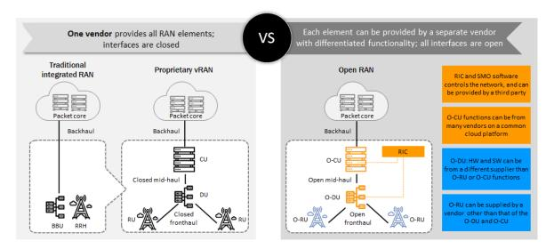
Figure 1. Disaggregation and open interfaces in Open RAN vs Traditional RAN
