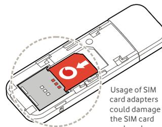
Usage of SIM card adapters could damage the SIM card card reader.
